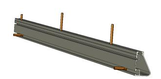
4. Attach this first piece of rail to the feet mounted on the roof. Mount the rail to each foot with a flange nut and hex bolt. Hand tighten the nuts and check the level of the rail.
