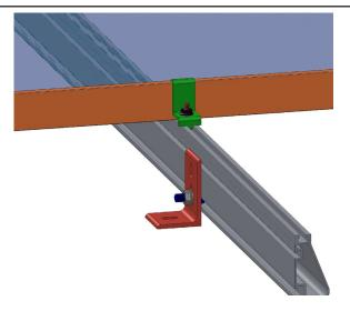
5. Working from the opposite side of the PV module. Assemble the center clamps by putting a clamp on the bolt, followed by the flange nut.
