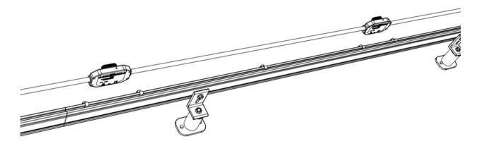
**NOTE**: Many PV modules have a central stiffening brace. In these cases, do **not** position the connector and microinverter at the exact center of the PV module, but position the Engage Cable so that the connectors do not conflict with the braces.
