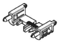
If the disconnect tool is not available, a #2 Phillips screwdriver can be used in its place. Insert the screwdriver into one hole, rock that side of the drop connector out, then insert the screwdriver into the other hole and pull the connector out entirely.
